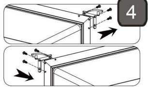
5. Remove the lower hinge supporter with the adjusting washer from right side. Install the lower hinge supporter in left side. Make sure to put the adjusting washers at the designated position.
